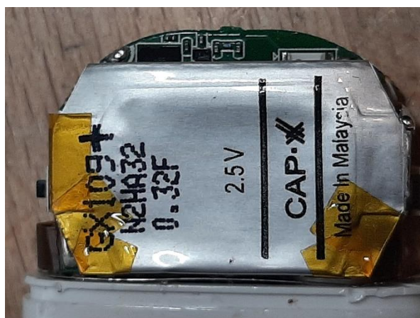
Kondensator (GX109+ N2HA32 2,5V / 0,32 F)
