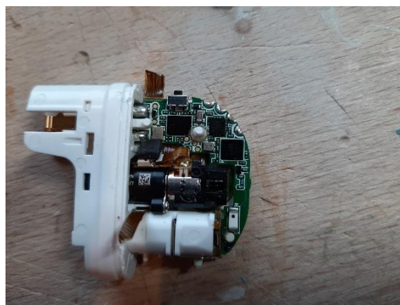
Kondensator (GX109+ N2HA32 2,5V / 0,32 F)
